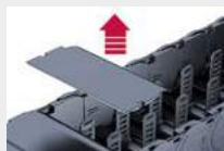
Detach the cover from the chain link
